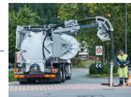
Combined suction and jetting hose boom KSR70
