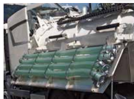
Hose rack - hydraulically tiltable via remote control
