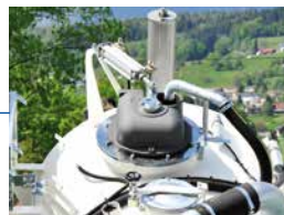
Suction/pressure changeover valve
